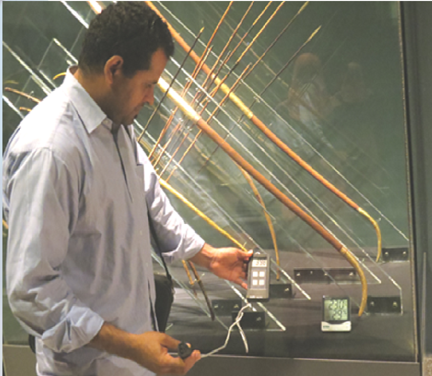
Measuring AT & (RH) by digital hygro-thermometer
